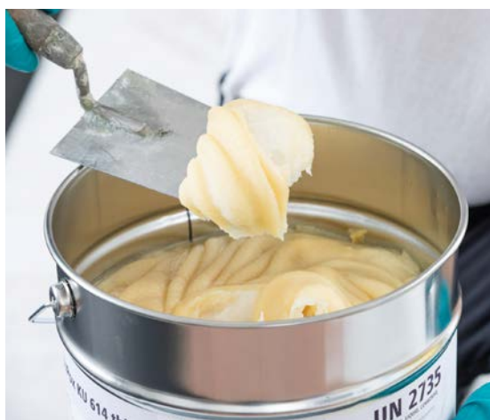
Component B is a pre-filled epoxy resin with which the surface structure is achieved. Photos left + title: Martin Baitinger
