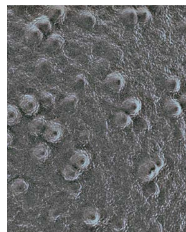
StoCryl V 700 coating surface with microtexture
